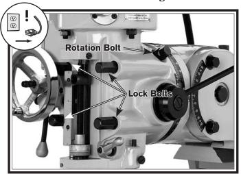
Figure 26. Head rotating controls.
